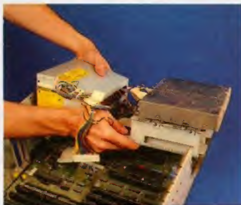
3 Removing the drive and power assembly is just a matter of undoing all the screws at the back and lifting it up. There is only a slot holding it at the front.
